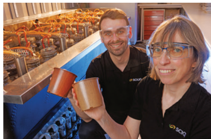
The PolBionix pots are made from biopolymers made from sugarcane, cassava or corn, combined with a biofiller of waste organic matter. Right: two of the Scion researchers who worked on the project, Maxime Barbier and Gerty Gielen
