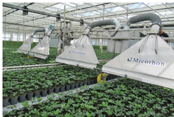
Original vacuum unit developed for a hellebore grower
