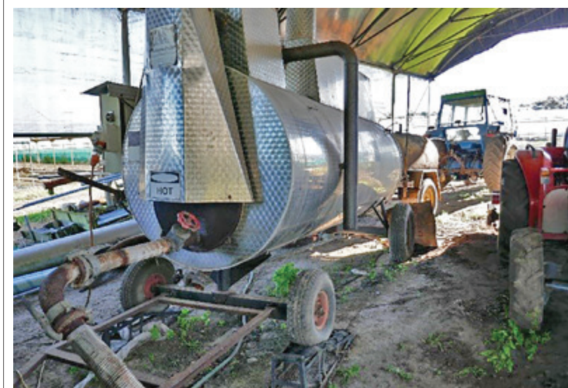
The mobile steaming unit – steam disinfection of media allows the next crop to be planted as soon as the mix has cooled, whereas fumigation with chemicals requires a four to six week wait
