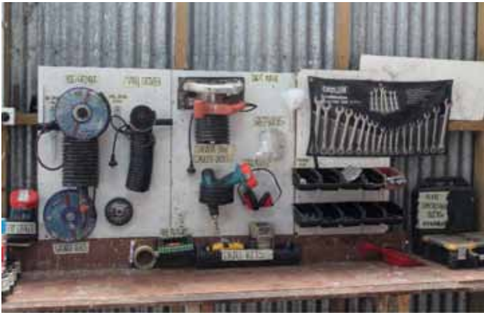
This tool cabinet has tools mounted vertically so people can see what's there. There is also a nearby re-stock checklist
